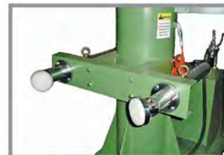
ADJUSTABLE TANK CENTERING DEVICE
