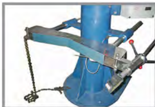
CHAIN / BELT CLAMP WITH TORQUE SWITCH
