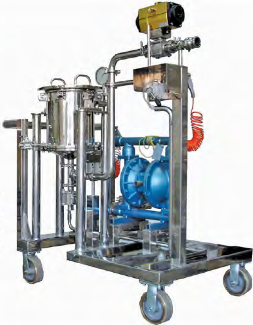
Filtration Skid : Diaphragm Pump with Cartridge Filter Housing
