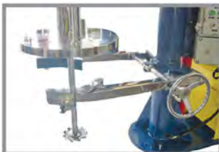
SCISSORS CLAMP WITH TORQUE SWITCH
